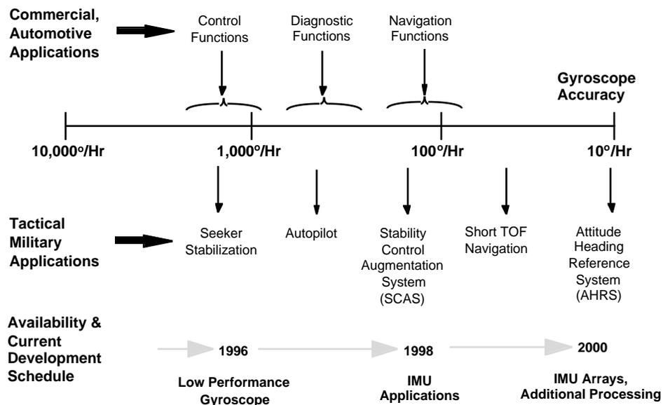
**FIGURE 7.** Overlap of Commercial and Defense Gyroscope Performance Specifications (adapted from data provided by Rockwell, Martin-Marietta, and Charles Stark Draper Laboratories).
